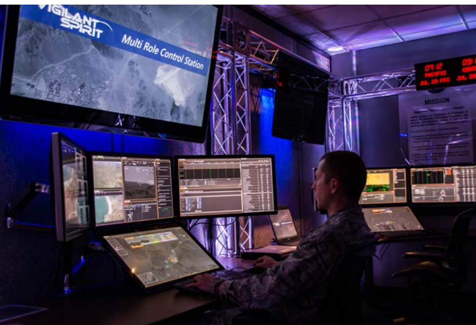
Captain Anthony Castello views the Vigilant Spirit Control Station at Wright-Patterson Air Force Base, Ohio. Engineers in the 711HPW's Supervisory Control & Cognition Branch developed the software which allows operators to control multiple UAVs at once. (Courtesy photo)
