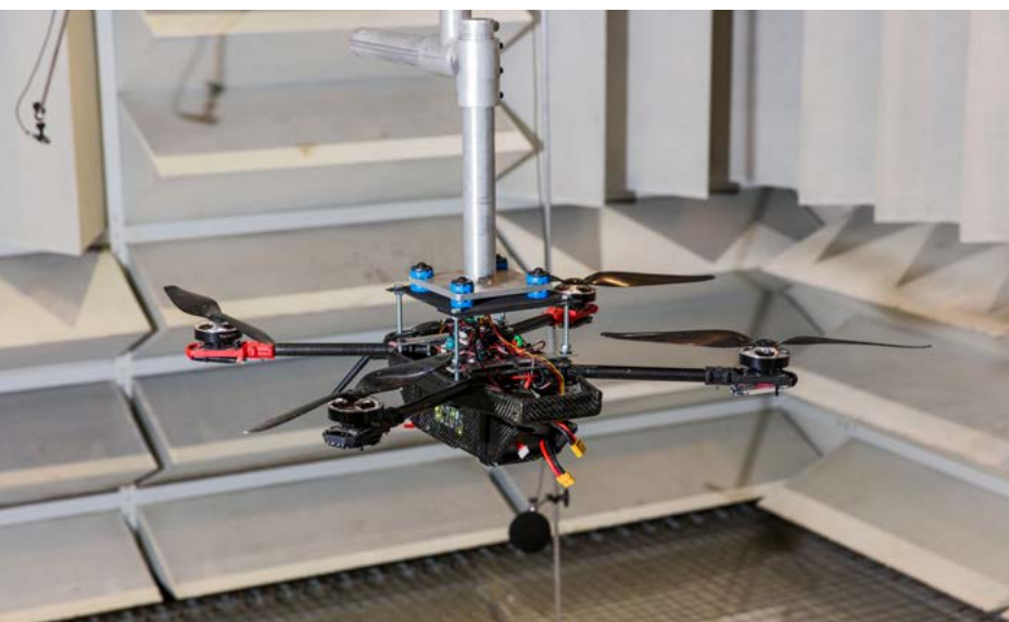
A small unmanned aerial system undergoes tests in the Acoustics Laboratory at Owens Corning Science and Technology Center in Granville, Ohio. (Photo courtesy of Owens Corning)
