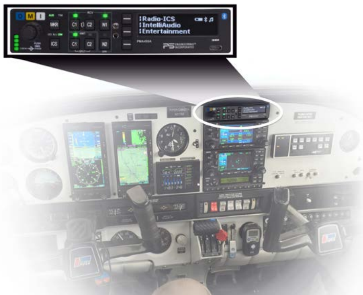
An installed PS Engineering PMA450A audio panel is shown. (Photo courtesy of PS Engineering.)
