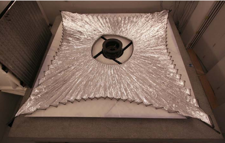
The Structure for Storing and Unfurling a Flexible Material (U.S. Patent 8,356,774), an Air Force owned invention, demonstrated in this solar technology. (Photo credit: AFRL/RVSV)
