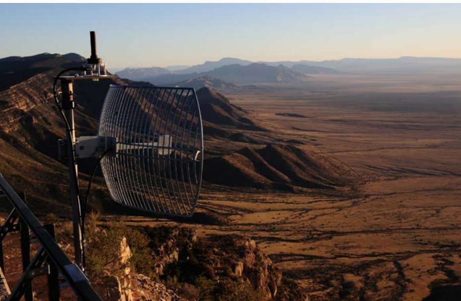
A LocataLite transmitter transmits high-accuracy positioning signals across the White Sands Missile Range, New Mexico, for testing methods developed for overcoming GPS jamming, or electronic warfare. This highly accurate navigation system was created through a Cooperative Research and Development Agreement between the Air Force Institute of Technology and the Locata Corporation. (Photo courtesy of Locata Corporation)
